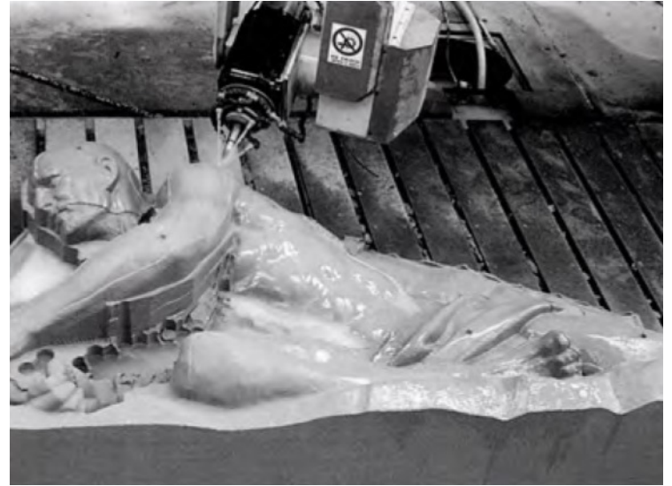
Robotic arm- blocking out
